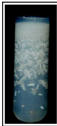
Fig 2. Dense precipitation and dendritic growth pattern obtained of cadmium oxalate in basic range
