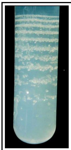
Fig1. Typical Liesegangring pattern obtained of cadmium oxalate
