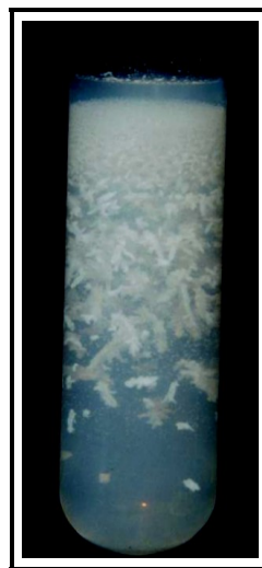
Fig 2. Dense precipitation and dendritic growth pattern obtained of cadmium oxalate in basic range
