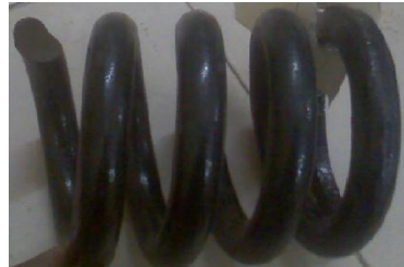
Figure 1. Photograph of failed coil spring having fracture surface.
